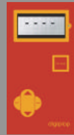
12. Unit is ready to measure. If you have introduced an offset, the display blinks.
