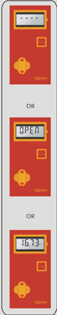
1. Normal measuring mode. Press "ENTER" to enter menu.
