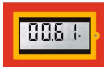
6. Measure again. Subtract the first measurement from this value. The result is the extension's offset.
