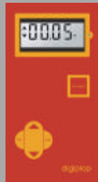
10. Editing offset Subtracts this value from the measured value, to account for extensions. Range: 0.0m to 0.5m
