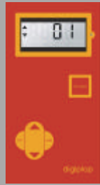
8. Editing the season. Season is set by setting the month. Month 0 disables the temperature gradient calculation. (S. Measurement theory) Range: 0 - 12
