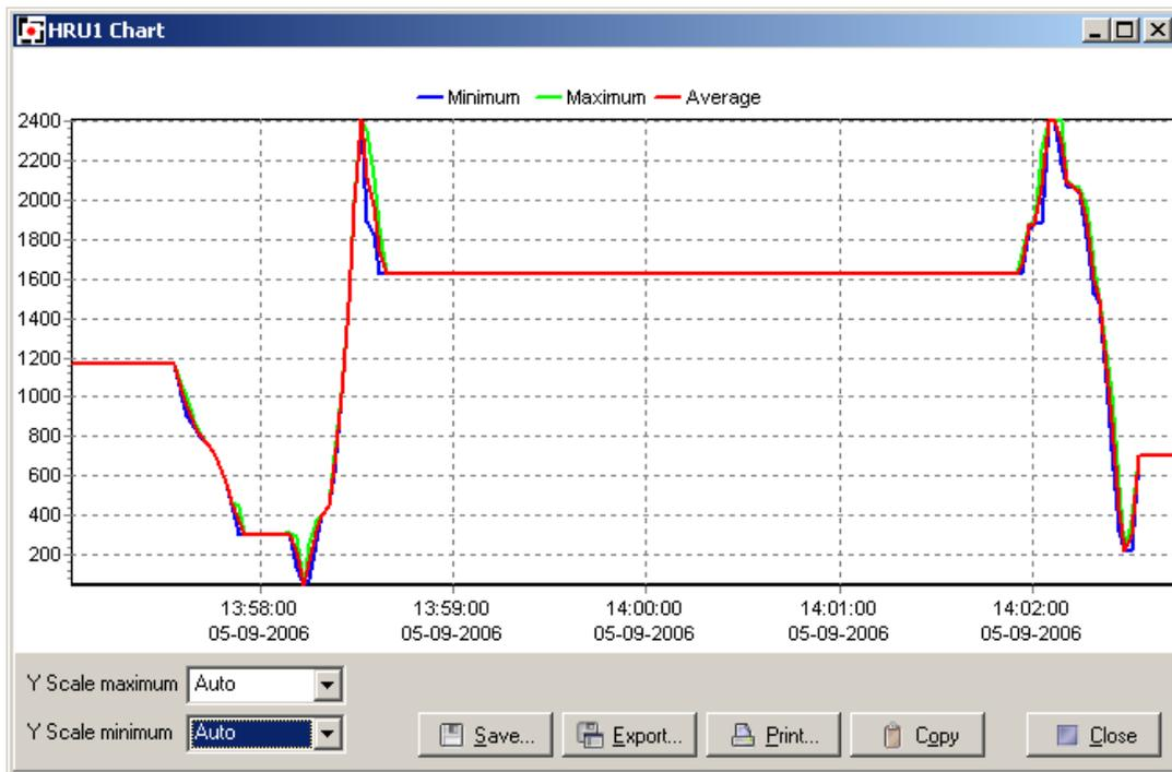
The Y scale can be manually set, and you can also use the mouse to zoom in on a specific area of the chart. Drag the mouse pointer from the top left corner of the area of interest, to the bottom right corner of the area of interest. When the mouse is released, the chart will zoom in on the selected area.
