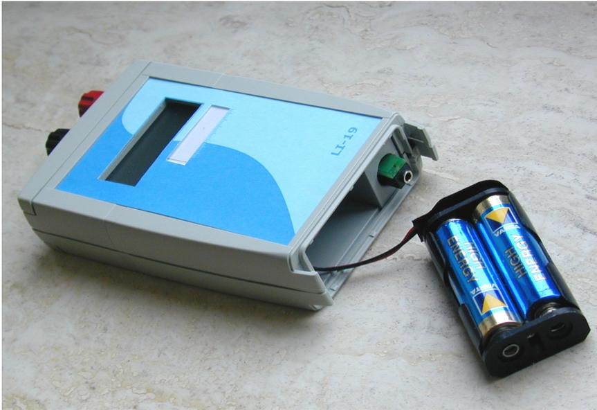
To prevent that the LI-19 is switched off while logging, the on/off switch is mounted so that the button has to be pressed quite deep to switch the LI-19 on or off. You can feel it and hear it when the switch toggles. Press the small black button far enough with your nail or a pencil until you feel and hear it switch.
