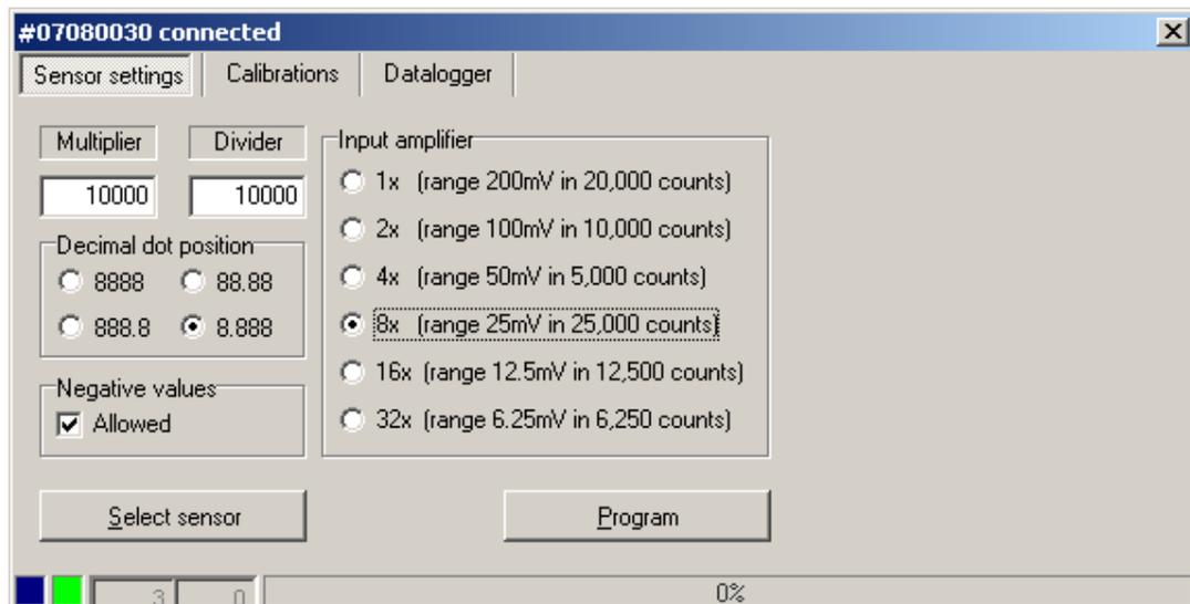
2. Next to the amplification factor, you can read how many internal counts each input range will give you. The number that the LI-19 should display at the full scale input value is entered into the multiplier input field. The number of internal counts that corresponds to that full scale input, is entered into the divider field.
